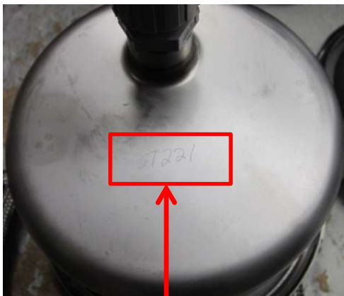
Single hub light housing, typically last fixture in the light set. Hand engraved.
